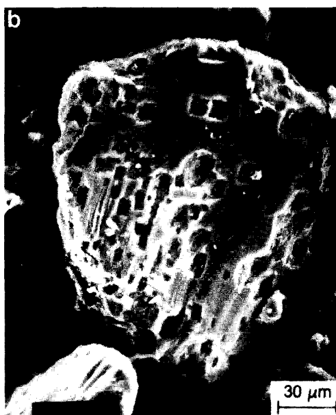
FIG. 3. SEM photo of Si particles before (a) and after (b) reaction with \text{CH}_3\text{Cl} in lab-scale fluidized bed for 4 h (Si utilizations 38%) using \text{Cu}/\text{Zn}/\text{Sn} catalyst at 300^\circ\text{C} .
